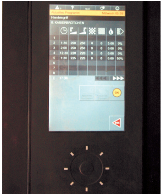
With the TC, baking parameters can be defined in several steps.
