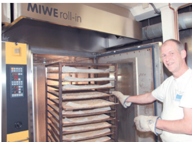
Loading the rack oven.
